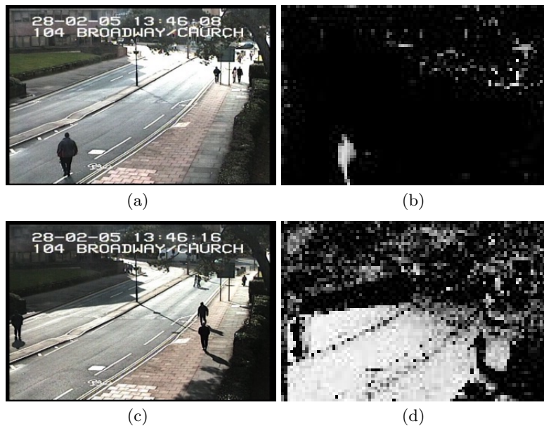
Fig. 1. Original frames (left column) and correlation-coefficient maps (right column), before (top) and during (bottom) an illumination change. The illumination change from cloud movement causes an increase in the correlation coefficient of a large number of pixels.
